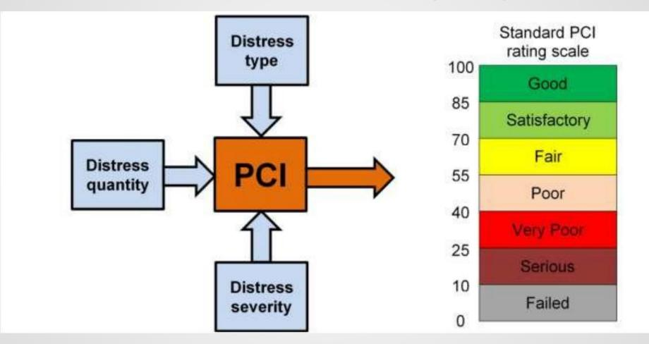
Rating scale used for Pavement Condition Index (PCI) Method (Shahin, 2005) https://www.researchgate.net/figure/Rating-scale-used-for-Pavement-Condition-Index-PCI-Method-Shahin-2005\_fig1\_337186891
